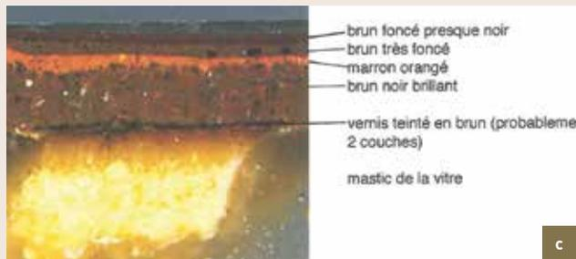
*L'Âne/Den Ezel*. a, b and c) Stratigraphic sampling and macro photograph of a window frame indicating an original layer of varnish (a and b) © M. Decroly, 2002; c) © KIK-IRPA, 2002).
