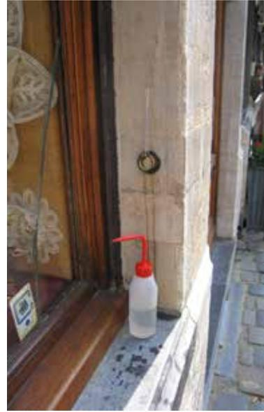
*L'Âne/Den Ezel*. Water absorption test with Karsten tube (© HHU, 2002).
